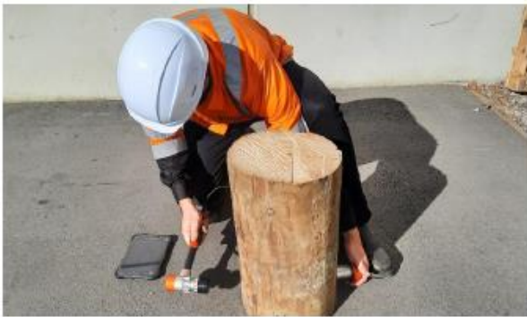
Suggested Body positioning for one knee down and other knee supporting geophone arm.
