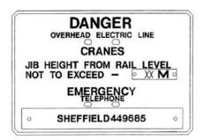
The crossing plates shall be mounted on concrete posts positioned on railway property near the boundary and under the centre of the power line. They shall be fixed at each side of the crossing except at single line tracks where only one sign shall be fitted.
