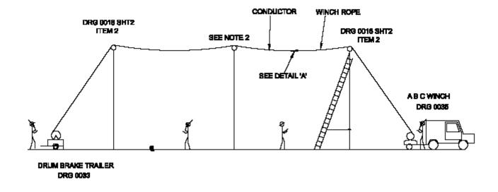
Further guidance for ABC conductor stringing can be found in drawing 1.09.145.0021, sheet 2
