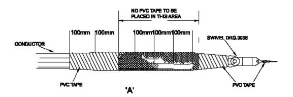
In all cases of stocking usage, the open end of the stocking shall be securely taped to the conductor to eliminate the premature release of the conductor stocking. Details of approved ABC and bare wire stockings can be found on drawing 1091450015 sheets 1 & 2.
