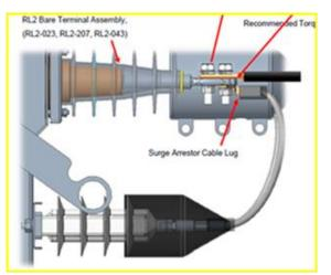
Typical arrangement for surge arrestor connection kits and associated shrouds:
