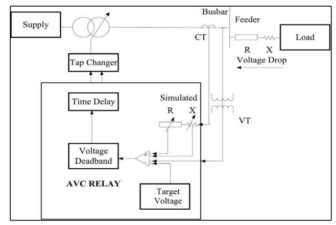
Figure 3: AVC scheme with line drop compensation operation<sup>6</sup>
