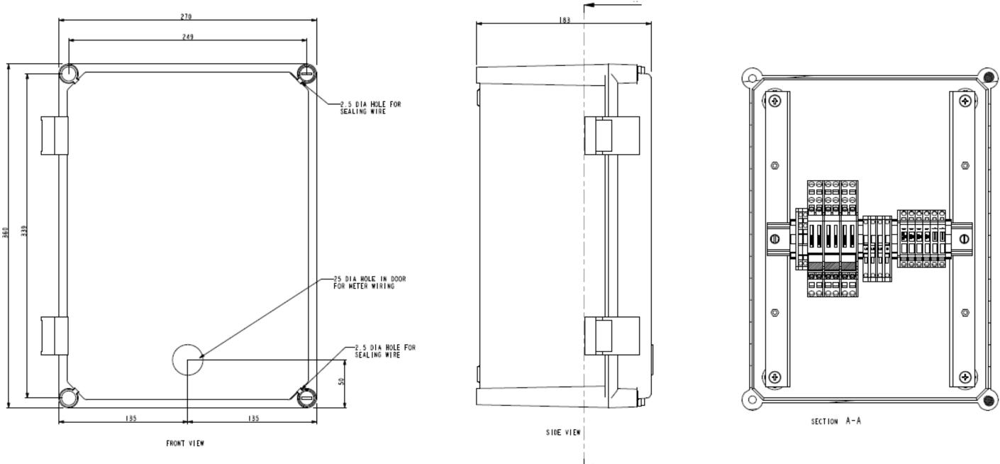
Appendix 8 - Metering Base/Panel Unit for CoP 5 Arrangement – Typical Example
