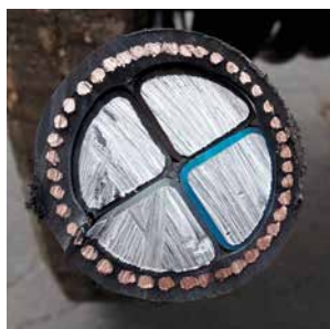
Figure 4: The inside of a LV 300mm 2 cable used to reduce losses on our network
