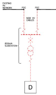
b) The Minimum Scheme is as for scenario a) above but the Customer requests an enhanced connection arrangement where the substation is looped into existing HV network.
