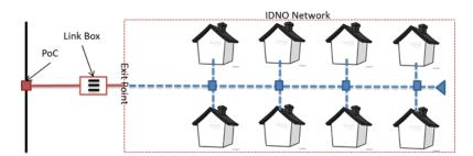
Where an ICP/IDNO is not able to insert fuses dead in accordance with figure 1 above, then IDNO/ICP must still install the fuses dead but then fit an insulated end at the boundary of the IDNO site before making the live final closing joint to the existing Northern Powergrid network, figure 3 sets details this arrangement;
