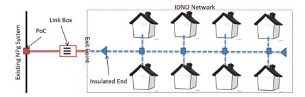
In instances where an ICP/IDNO requires fuses inserting/removing from a Northern Powergrid owned link box, it must request the relevant Northern Powergrid project engineer to attend site and
