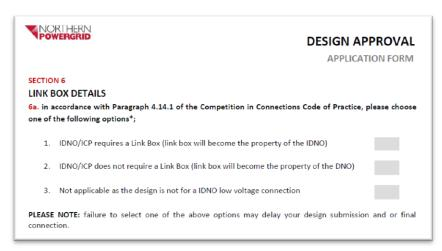
In addition, as part of our minimum requirements for design submission, the scaled approval drawing must indicate the proposed ownership details. Where this information is not provided, this may result in a design submission being rejected.
