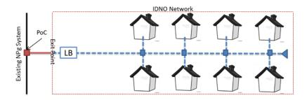
Northern Powergrid will have the right for operational access of the ICP/IDNO owned link box under emergency situations and for the purpose of isolating a fault on the IDNO network which may be disrupting Northern Powergrid customers in accordance with Engineering Recommendation G88/2.
