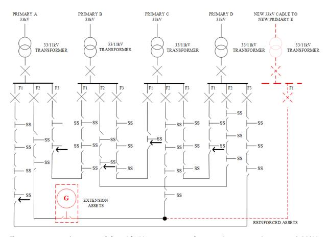
The existing network consists of four 10MVA primary transformer substations and associated 11kV switchgear. A new connection of 4MVA has been requested in the vicinity of F2 from Primary A.
